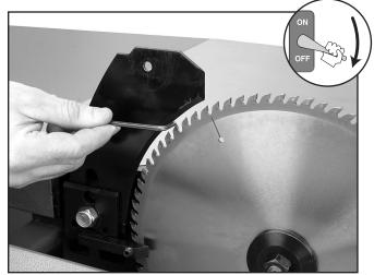
Figure 40. Aligning the riving knife.
